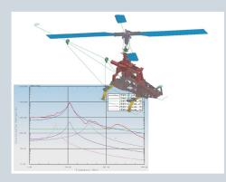
motion and distributed loads (e.g., dynamic pressure). The user can then apply excitations to the structure, controlling dynamic modes, static corrections and damping assumptions to define an event for analysis. Motion, force and stress responses can be predicted as either XY plots at specific locations or as contour results over sections of the model or the complete model. Strength and peak results can be generated for elements by
